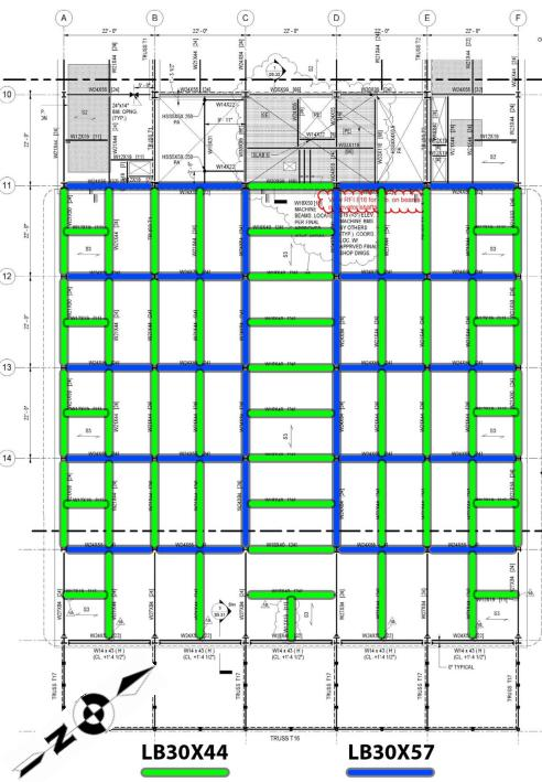
Figure 5.12: Cellular Beam Layout
